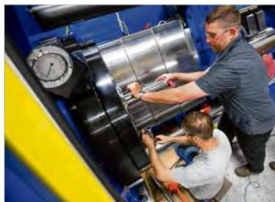
Builder Jeff Feltz, left, and manufacturing supervisor Cory Smith work on a 300-ton rotary friction welder on Friday at Manufacturing Technology Inc. in South Bend.
