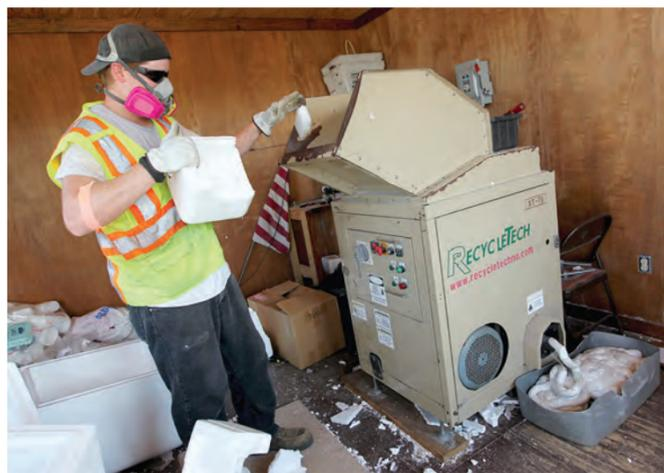
Charles Coulter feeds recycled foam containers into the multiple foam densifier at Galveston's ECO Center.
