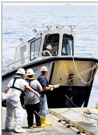
Crew members guide a mumson boat off of the deck of the Pacific Responder oil skimming vessel on the Gulf of Mexico on Thursday. The boat ties up to a boom trailing behind the responder, and then the two pull the boom to contain oil leaking from the Deepwater Horizon oil wellhead.
